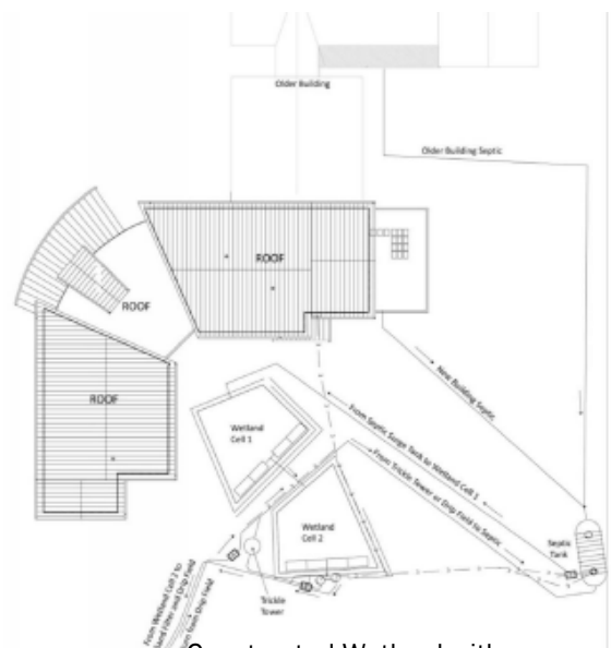
Constructed Wetland with tank, trickle system and piping.
